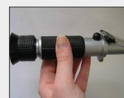
Hand-held salinity refractometer ACC100
