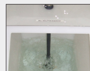
Salt solution tank fitted with air agitation ACC59/6
